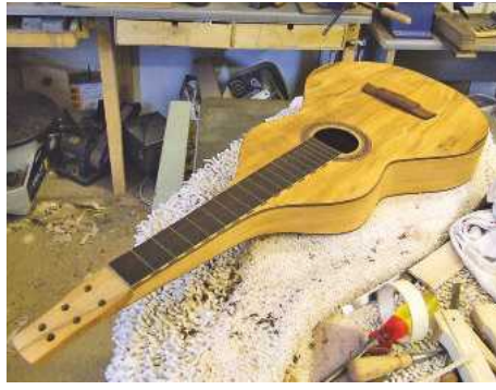
▲ Pic.28 The coat of oil was applied and wiped off after five minutes. Six coats of shellac were then applied
